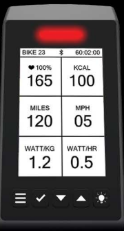
DISPLAY 02 Shows the user's further detailed "actual" performance data such as heart rate, watt / KG and watt / HR.
